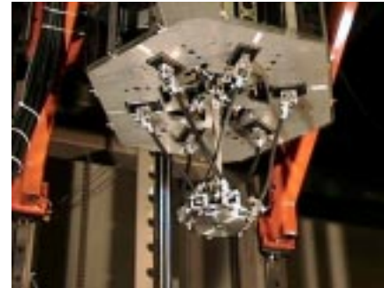
ParaDex prototype closed-chain manipulator being investigated for force-guided mechanical assembly
