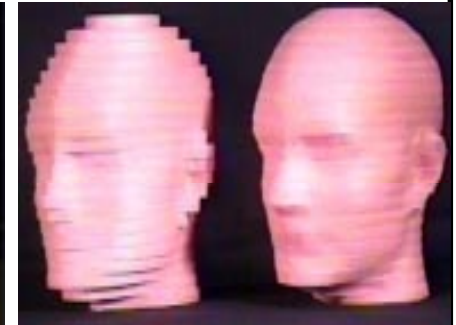
Vertical cut vs. tangent cut 3-D objects fabricated by CAM-LEM solid freeform fabrication system
